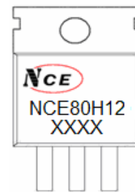
Marking and pin assignment
